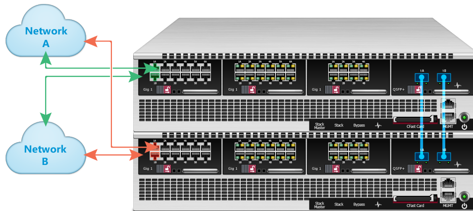
Figure 6. TippingPoint NX Series IPS – two-device stack with multiple network segment devices
