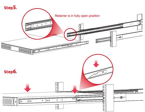
Press trigger down to release the slides from locking
