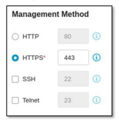
The HTTP and HTTPS protocols are used for connecting to the web management console. The SSH and Telnet protocols are used for connecting to the CLI commands.
