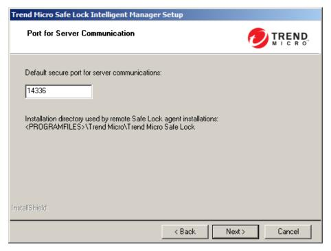
FIGURE 3-7. Setting the Server Communication Port
