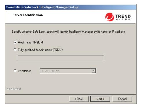
FIGURE 3-5. Configuring the Server Identification
