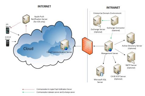
FIGURE 1-1. Enhanced Security Model with Cloud Communication Server
