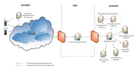
FIGURE 1-2. Enhanced Security Model with Local Communication Server
