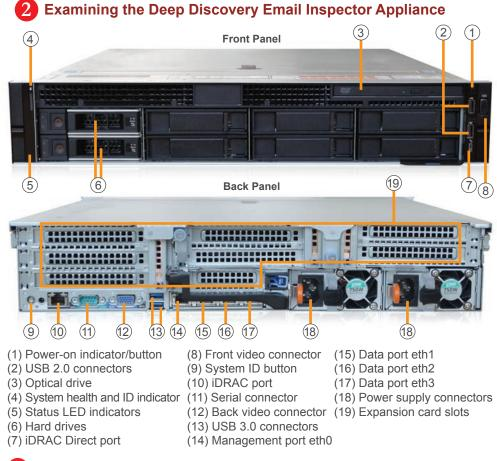
Note: Your device comes with the Copper Ethernet NIC. If your purchase includes the optional 1Gb Fiber Ethernet NIC, install it in the full-height expansion card slot. If your purchase includes the optional 10Gb Fiber Ethernet NIC, install it in the half-height expansion card slot.
