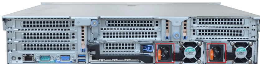
FIGURE 3-2. 1200 appliance AC power slots
